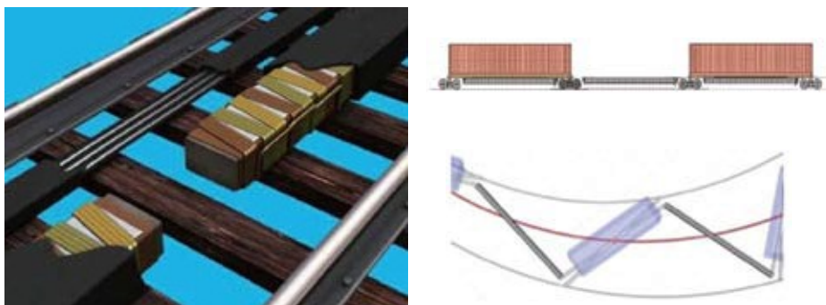
Figure 2_ LIM-type driving gear and the shape of linked wagons
